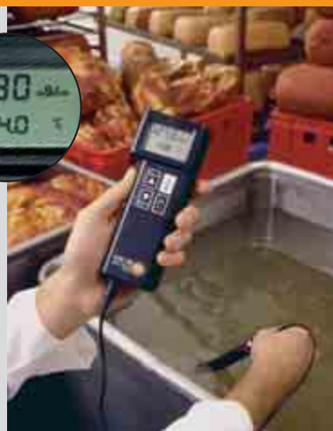
Measuring salt level (NaCl) in pickling brine
