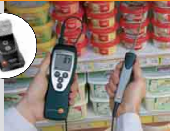
Inspects a refrigerated counter for sufficient refrigeration power
