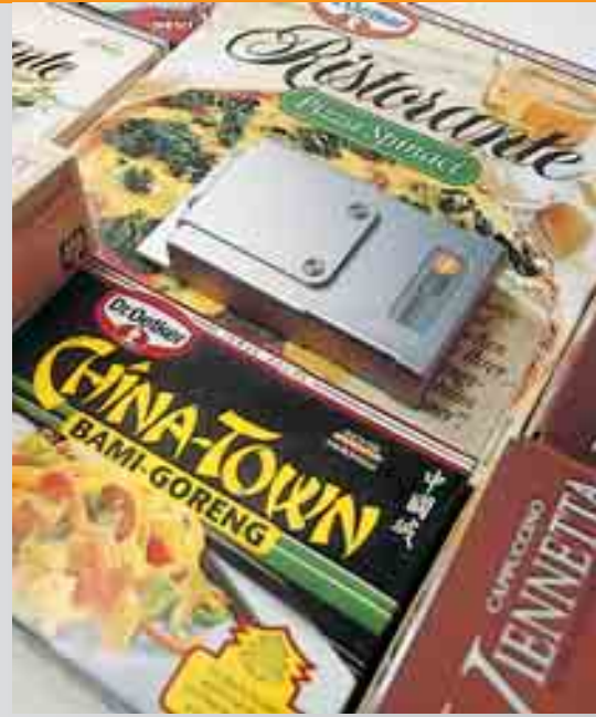
testostor 171-0 monitors fluctuations in temperature constantly
