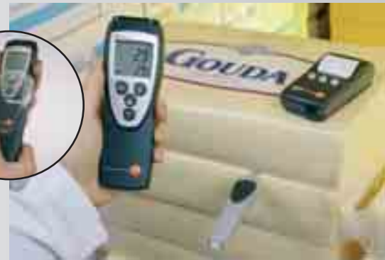
Practical monitoring during cheese storage, wireless, measurement data transmission via radio
