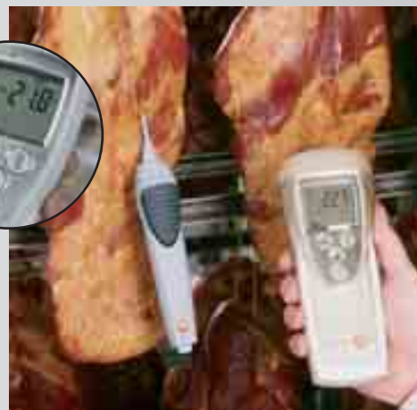
Measurement of penetration temperature when smoking foods, wireless radio transmission of measurement data
