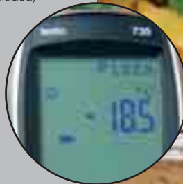
Displays site and parameter. Up to 99 product names can be stored in the instrument
