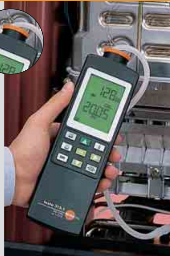
Checks gas flow pressure
