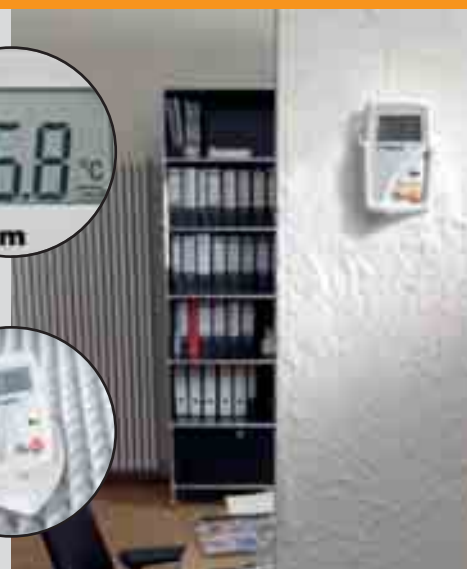
Logging room temperature with immediate alarm display if limits are exceeded
