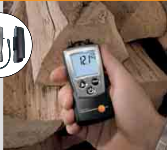
Fast and easy wood moisture measurement
