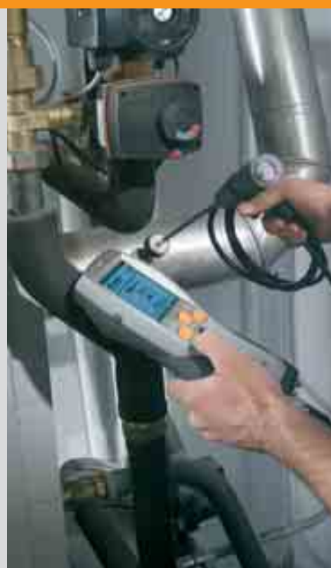
Flue gas measurement in a burner
